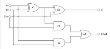
Figure 5: Full Adder Circuit
