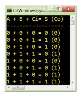
Figure 8: Full Adder Implemented as TDF Network Demo Result
