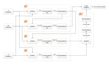
Figure 6: Full Adder Implemented as TDF Network
